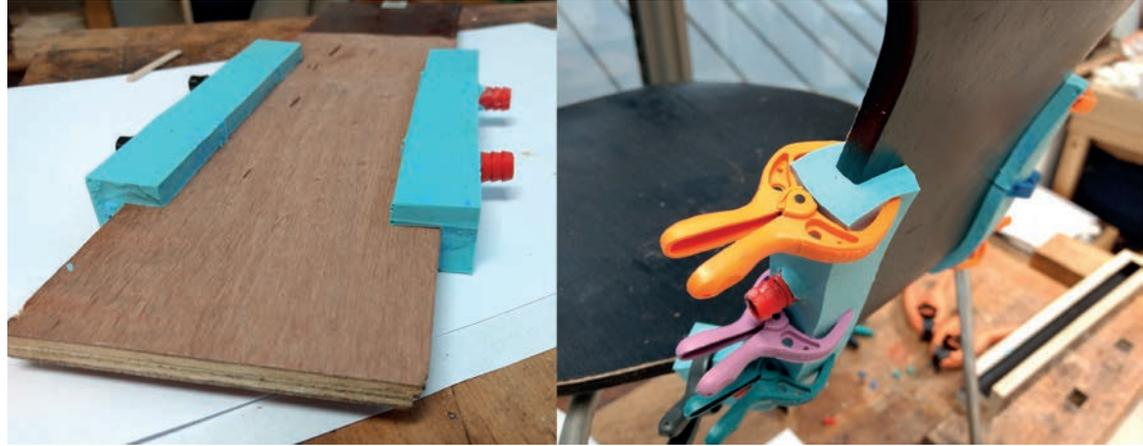
the delaminated area (figures 7a, 7b). It is best described as a mouthpiece with an inlet and an outlet. The silicone rubber was cast and proved to be a re-usable and flexible component. This made it easier to set up the testing rig and to remove the components after infusion. With these silicone mouthpieces double-inlet and -outlet valves were tested. A better spread of the adhesive was expected but in practice it had the same results as with the previous vacuum compartment.
