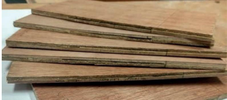
Figure 4 Delaminated plywood mock-ups.
