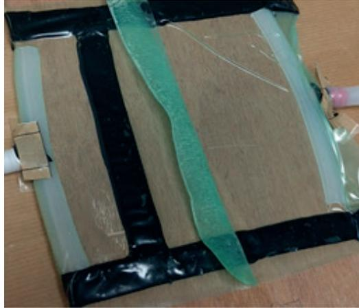
Figure 5 Vacuum compartment with mock-up, PE film, tube connectors and sealing tape.
