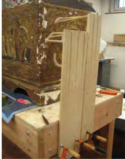
Figure 19 Applying pressure to new cast ornament with custom-made clamping setup.
