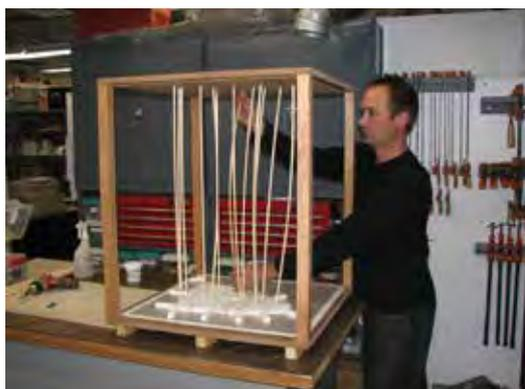
Figure 16 Shimbari frame with wooden go-bars to register fragments during reassembly.
