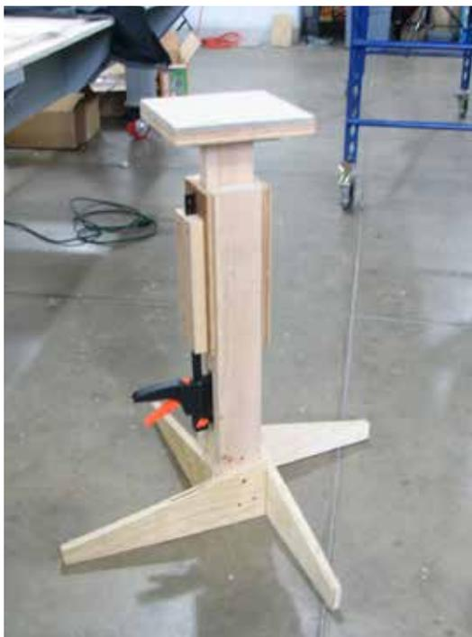
Figure 24 Adjustable counter support for lacquer panel.
