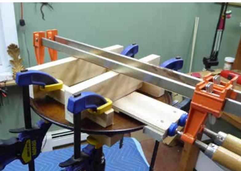
Figure 2 Tripod table clamping setup.
