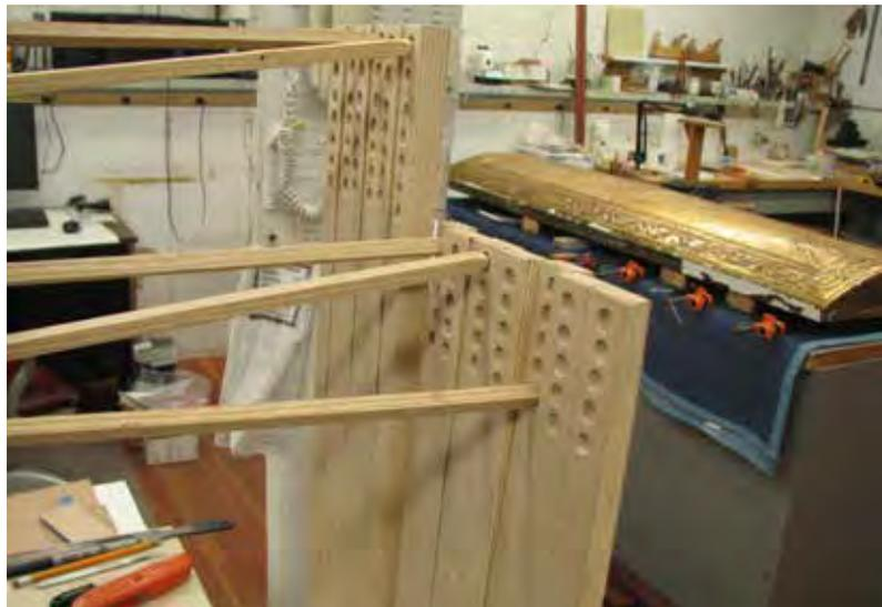
Figure 20 Registration holes for go-bars.
