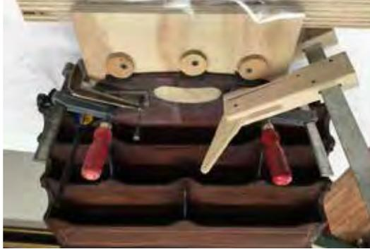
Figure 4 Circular discs with off-center screw fixture.
