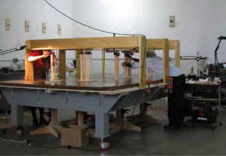
Figure 22 Clamping table setup with bridges allowing targeted pressure.
