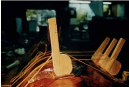
Figure 5 Cam-action toggles on bombe chest with marquetry.
