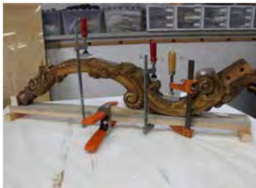
Figure 12 Gluing a shear break on a serpentine leg.
