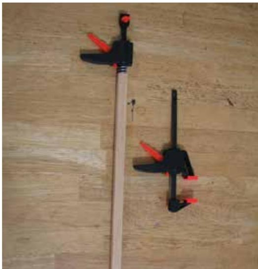
Figure 23 Reconfigured mini-bar-clamp used as a spreader/go-bar on clamping table.
