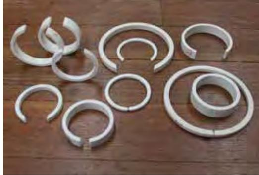
Figure 9 Spring clamps sliced from PVC piping.
