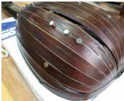
Figure 21 Earth magnets holding staves in place during hide glue curing.
