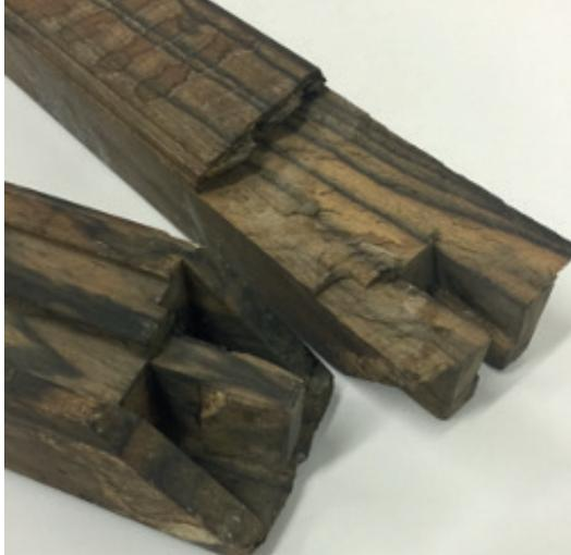
Figure 6 Detail of the broken top right corner joint.
