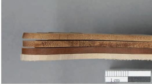
**Figure 4** Varying degree of darkening of ornament cut edges (maple veneer 2.5 mm). From top to bottom: CO<sub>2</sub> laser (pw), CO<sub>2</sub> laser (cw), frequency-tripled Nd:YAG laser, hand sawn.
