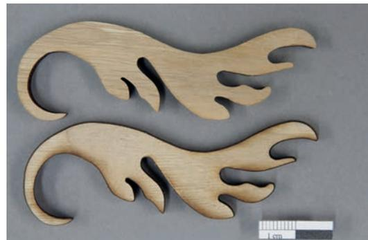
**Figure 6** Top surface darkening (walnut veneer 6 mm). Top: CO<sub>2</sub> laser (cw); bottom: CO<sub>2</sub> laser (pw).
