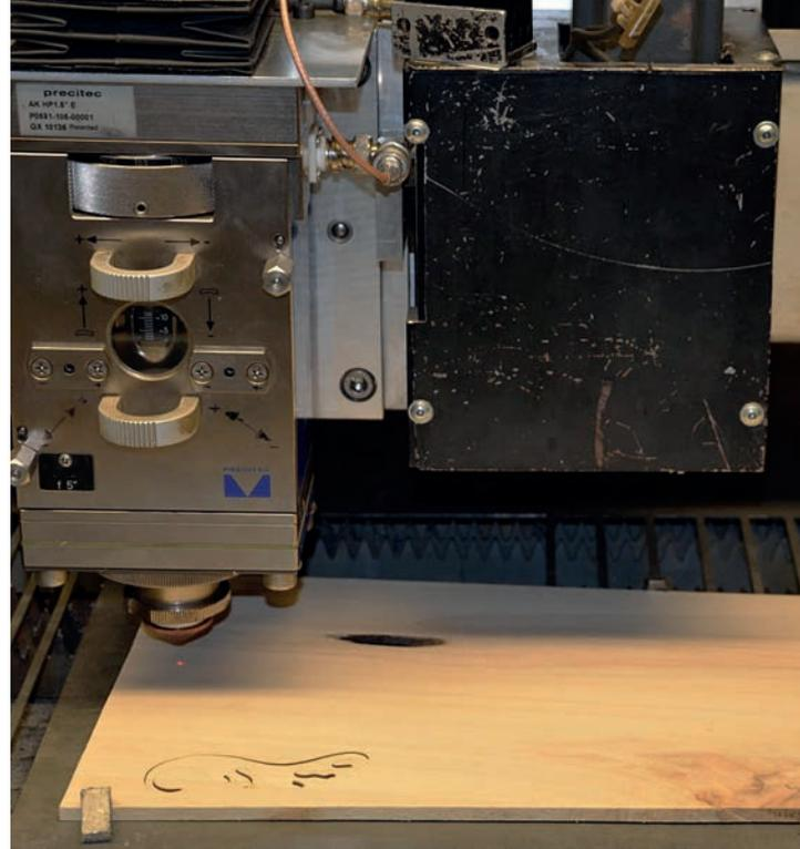
Figure 3 Cutting head of the CO<sub>2</sub> laser (cw).
