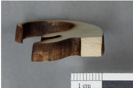
**Figure 5** Cross-section of an ornament (maple veneer 6 mm) cut with the CO<sub>2</sub> laser (pw).
