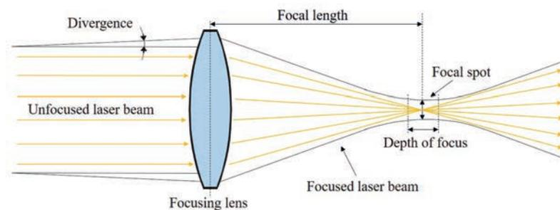
Figure 1 Schematic diagram of a focused laser beam.
