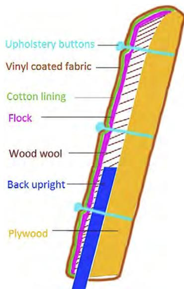
**Figure 6** The structure of the upholstered back support of the Artek chair.
