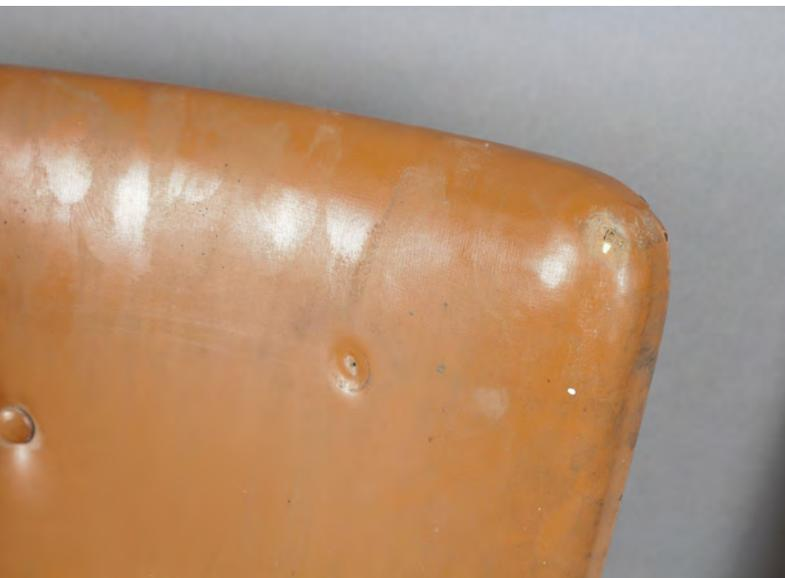
**Figure 7** A thick layer of dirt had stuck onto the oily vinyl surface which was caused by the emigrating plasticizer.
