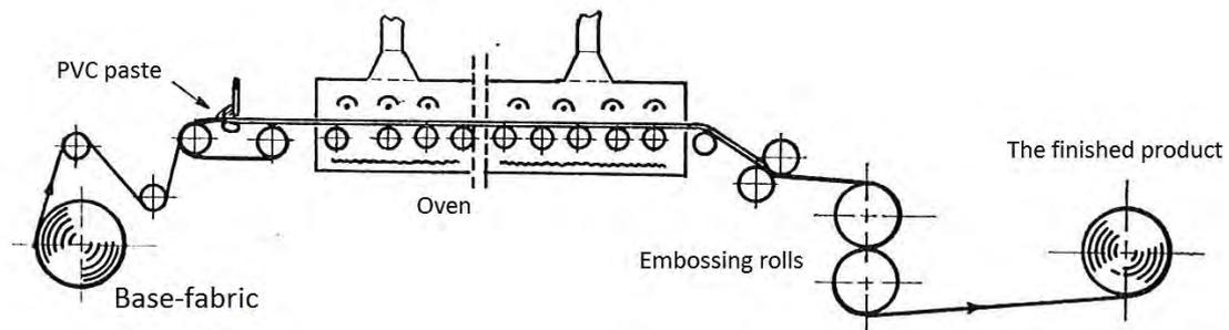
Figure 1 A coating machine (A. Kulju, *Muovien teknologia*, Porvoo 1965, p. 283).
