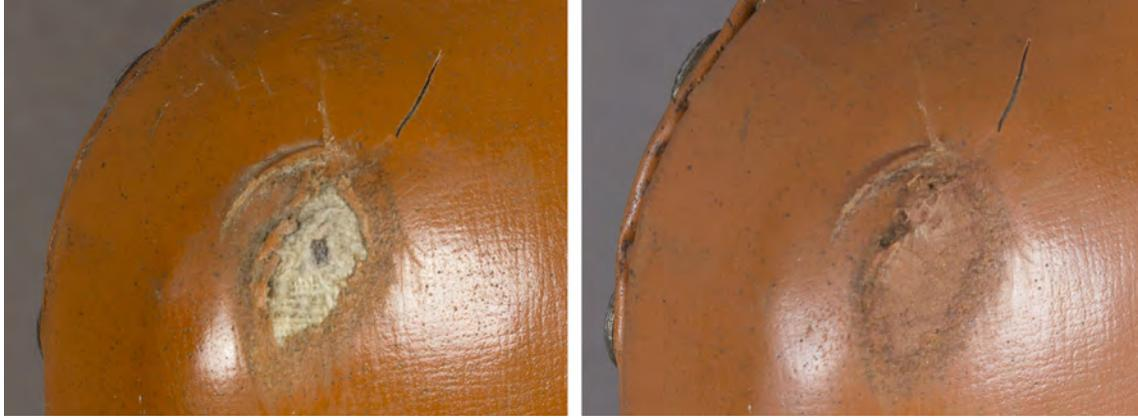
Figures 8a, b A hole in the vinyl fabric before and after conservation. The fill was prepared with Laropal A81, pigments and hollow glass microspheres to imitate the damaged and matte vinyl.
