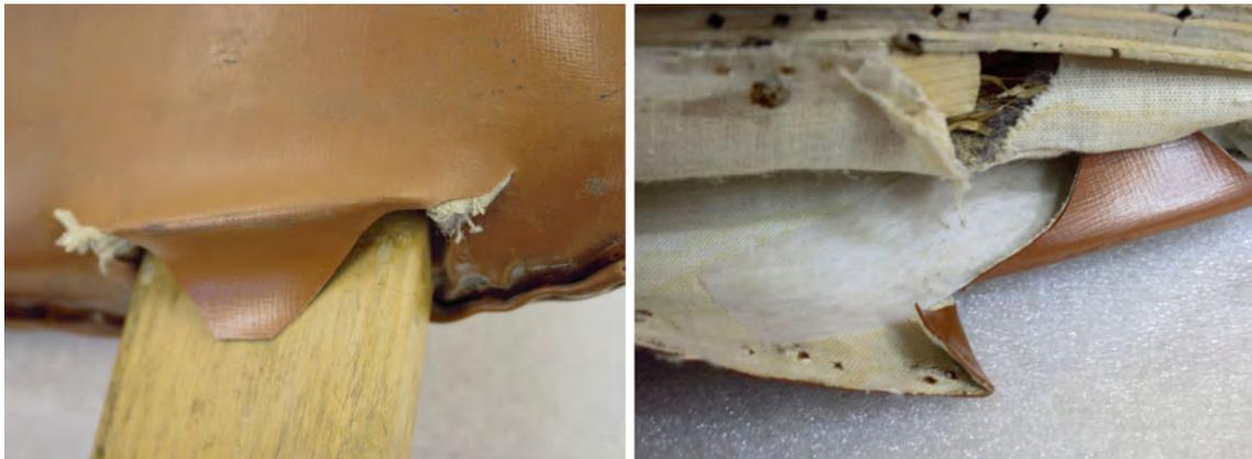
Figures 9a, b The tears of the vinyl were supported with Reemay.
