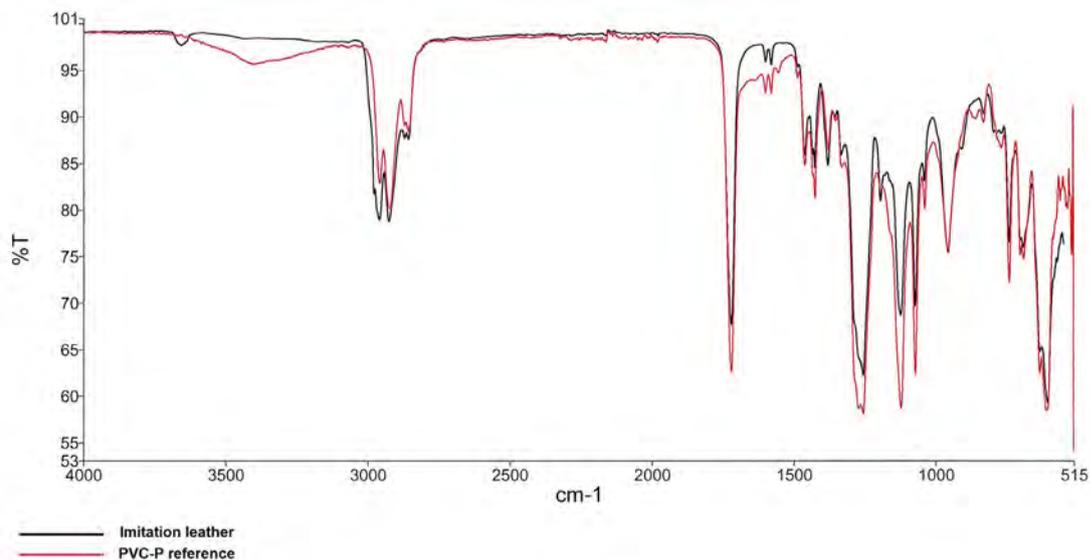
**Figure 3** The FTIR spectra of the imitation leather of the Artek chair and the PVC-P reference clearly indicated that the imitation leather had a PVC coating.
