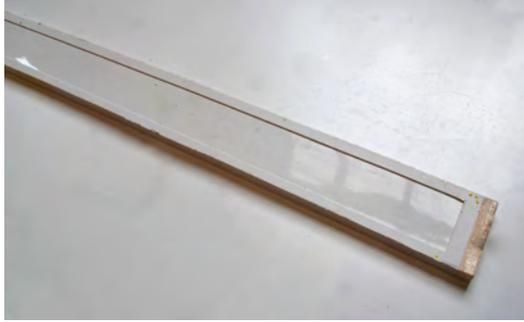
Figure 5 A silicone rubber mould with a 1 mm deep impression.
